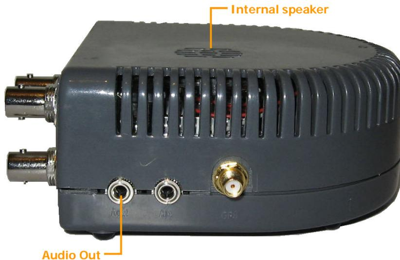
*Figure 22: Internal speaker and Audio Out connector*
