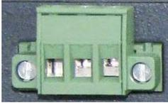
**Figure 33: Wire connector plugged into Power connector**
