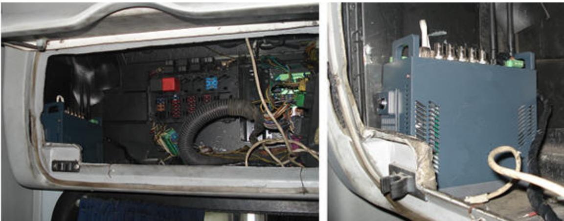
**Figure 4: Video Gateway installed in the compartment above the driver's seat in a bus**
