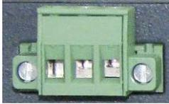
**Figure 30:** Wire connector connected to Power connector
