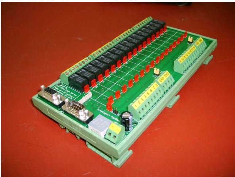
**Figure 20: IA 3126-2 relay board**
