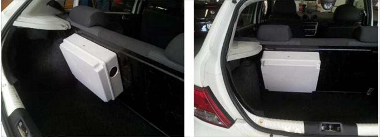
**Figure 2: Video Gateway installed in an insulated container and attached to the back of a seat in a car**
