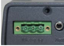
Figure 28: No wire connector connected to Power connector
